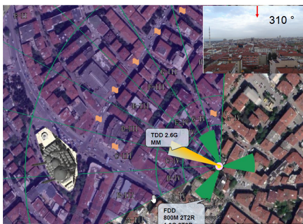
FIGURE 3. Location and azimuth angles of the experimental massive MIMO test environment.
