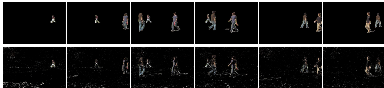
FIGURE 6. Selective subtraction as background subtraction: The results of the proposed selective subtraction method when the reference plane is the far wall and hence all moving objects are considered foreground as in traditional background subtraction techniques. First row shows the results obtained from the proposed method and the second row shows the results from state of the art mixture of Gaussian method [6]. The results indicate that the proposed technique can be used as background subtraction and gives better qualitative results.
