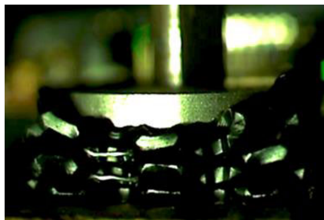
FIGURE 10. High-Speed video of two different drop tests: 50 mm [1 m/s] (A), 100 mm [1.4 m/s] (B). The frame in each case shows the moment of maximum compression [47].
