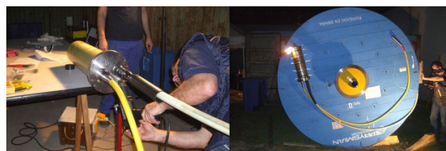
FIGURE 4. Left: Termination box. Right: Cable deployment with termination box unit.
