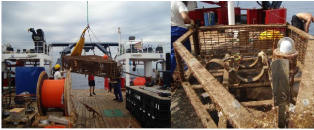
FIGURE 11. A. OBSEA on board R/V Sarmiento de Gamboa. B. A close up view showing the dome and the camera.
