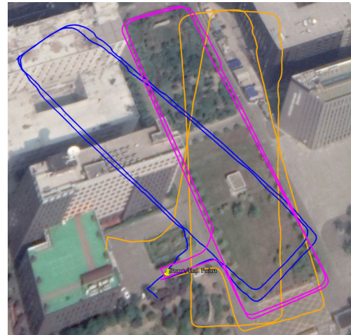
FIGURE 22. Pedestrian test plane projection trajectory on Google Earth. The brown line indicates only using ZUPT algorithm, the blue line indicates using ZUPT +iHDE (the method used in literatures), while the magenta line indicates using ZUPT + proposed heading constraint algorithm.
