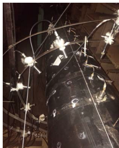
(b) Experimental layout of the sensing fiber
