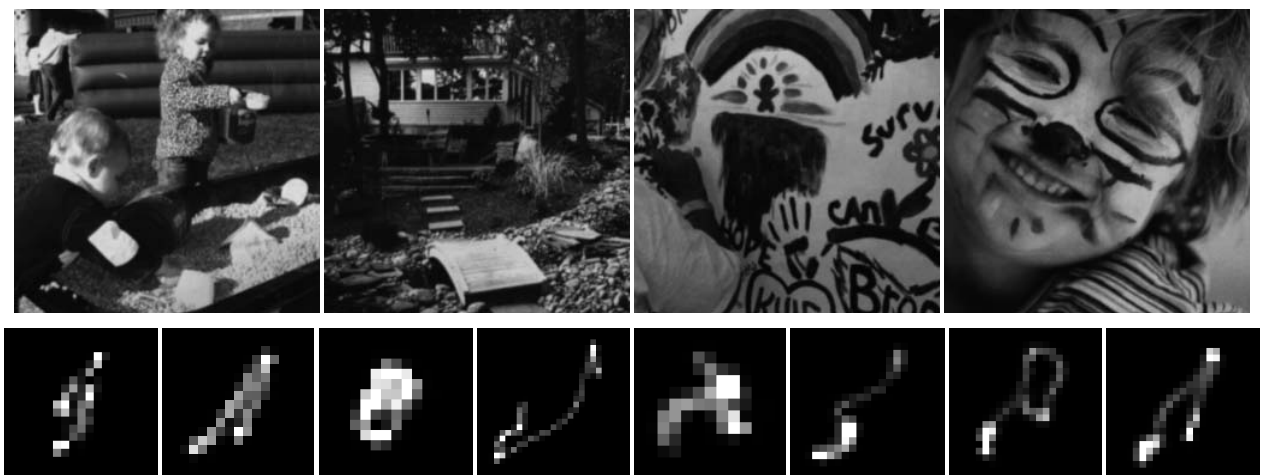
FIGURE 8. Ground truth data: 4 images and 8 blur kernels, resulting in 32 test images.
