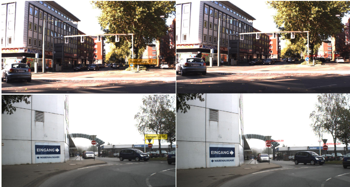
FIGURE 12. Traffic sign detection results in GTSDB. The detection results of cascaded R-CNN network are shown on the left, and the results of network with our proposed method are shown on the right. Especially, one target of images in the second row is undetected and another is false detected using the cascaded R-CNN network on the left while they are both detected on the right.
