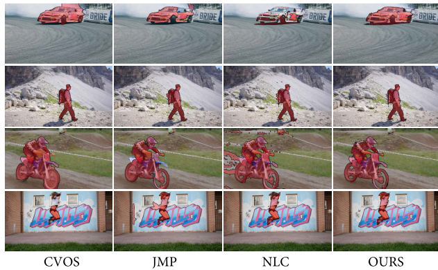
FIGURE 1. Segmentation results of representative frames in 4 sequences for four methods (From left to right: CVOS [9], JMP [25], NLC [17] and our method). We can see that the three compared methods may produce accurate segments in some sequences, but may perform poorly in others. By contrast, our method achieves superior results in all situations. (Best viewed in color).
