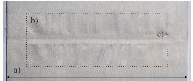
FIGURE 12. A photograph of the insulation paper sample at parameters values A1, B1, C1, and D1 : a) Paper width = 71 mm, b) Paper in the slot = 55 mm * 21 mm, c) Pinhole after the breakdown voltage V_B test.
