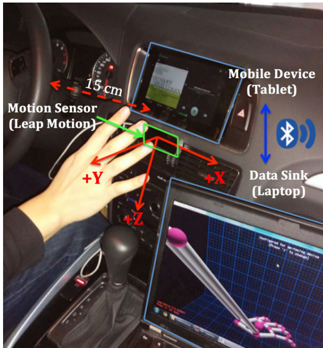
FIGURE 1. The in-vehicle experiment setup. A laptop is used for gesture recognition, visualization and controlling. The Leap Motion sensor is connected to the laptop via USB 3.0, reporting hand positions. The mobile device (tablet) is connected to the laptop via Bluetooth and being controlled.
