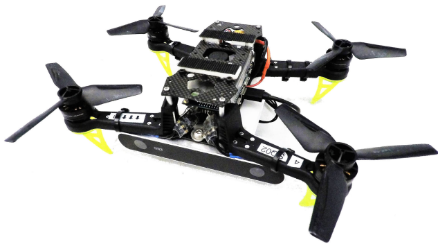
FIGURE 5. Detector drone platform used in the experiments. It is equipped with a ZED camera, a Jetson TX2 (used for perception) and a Snapdragon Flight board (used for control).
