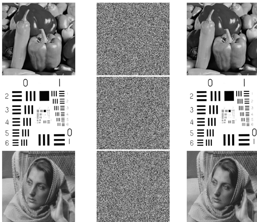
FIGURE 5. (continued.) The simulation results of the proposed cryptosystem. The first column images are plain images, the second column images are cipher images, and the last column images are decrypted images.
