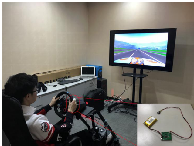
FIGURE 1. The driving simulator and the tactile vibrator (on his right hand as highlighted in the red circle).
