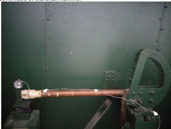
(b) Testing of sensor by Marshall hammer
