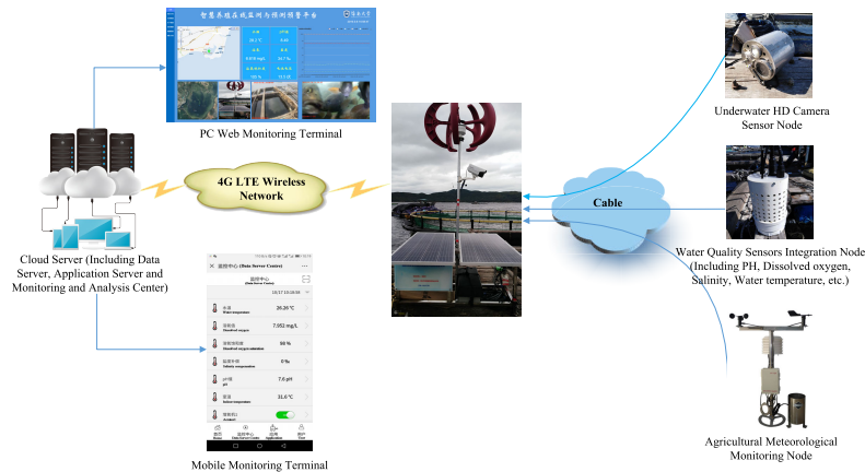
FIGURE 1. The topology structure diagram of the smart mariculture IoT system.
