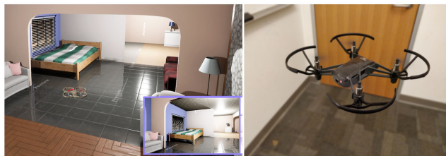
FIGURE 1. (left) DRL for autonomous navigation is carried out on a set of manually generated 3D realistic meta-environments. The learning is transferred to a new test environment and only last few layers are trained. (right) The approach is also tested in a real environment using DJI Tello.
