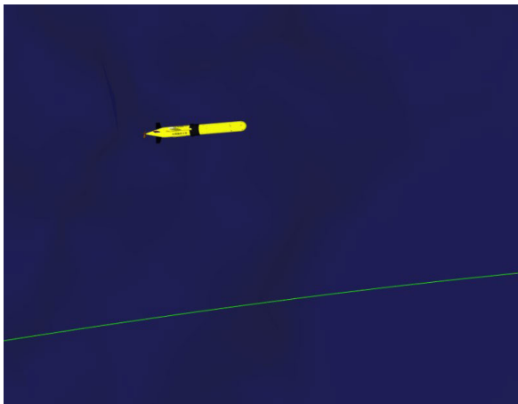
FIGURE 7. Human-machine interaction interface for displaying of the real-time attitude of AUV. Note that the solid green line represents target path.
