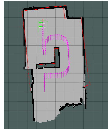
(a) Real-time position of the mobile robot recorded on the grid map.
