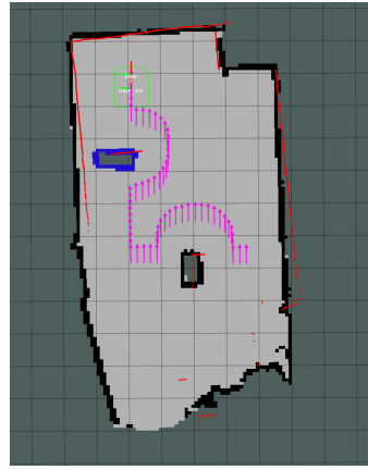
(a) Real-time position of the mobile robot recorded on the grid map.
