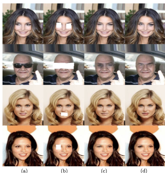
FIGURE 5. Comparisons of the model with skip-connection and the model without skip-connection in inpainting details.
