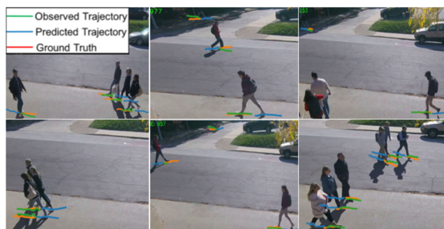
FIGURE 6. Illustration of our method predicting future 12 time steps trajectories, given previous 8 time steps ones.
