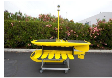
FIGURE 19. Wave-driven unmanned surface vehicle Wave-Glider.
