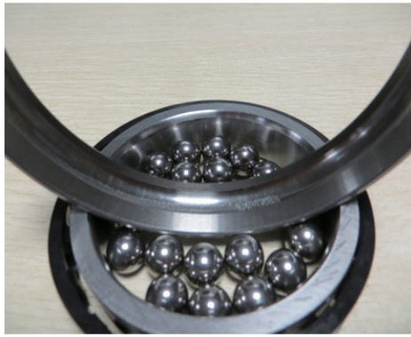
FIGURE 10. The local fault on the outer raceway.
