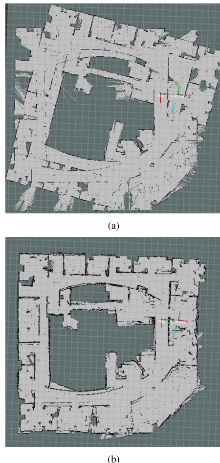
FIGURE 12. When the error of front-end is large, map built by RBPF (a) gradually rotated a certain angle for lack of global consistency.
