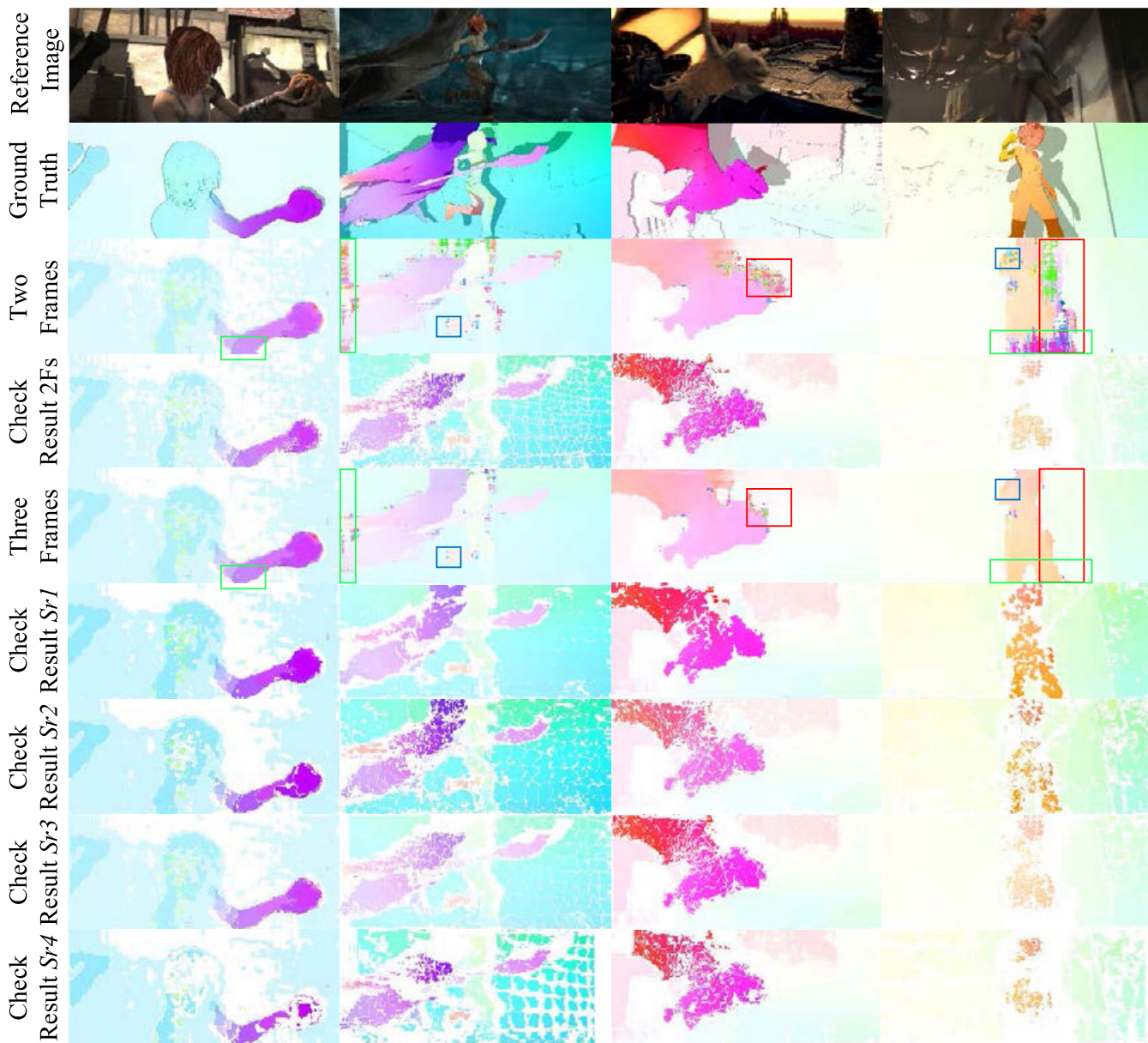
FIGURE 4. Optical flow results illustration: the first row illustrates the reference image; ground truth with occlusion mask (shadow area) is shown in the second row; the third row illustrates discrete optical flow using two frames; the two-frame approach results after consistency check is shown in the forth row; the fifth row illustrates the optical flow results with three frames; three-frame approach results with different outlier removal strategies are shown in the sixth - ninth rows.
