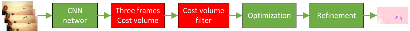
FIGURE 5. Proposed additional algorithm based on tripe image matching cost and cost volume filter: outlier handling and interpolation part are not necessary in this simplified pipeline.
