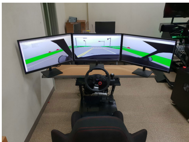
FIGURE 10. The experimental apparatus for human driver. A human driver can manipulate the steering wheel, gas pedal, and brake pedal and is available with the front, left and right view through 3 displays.
