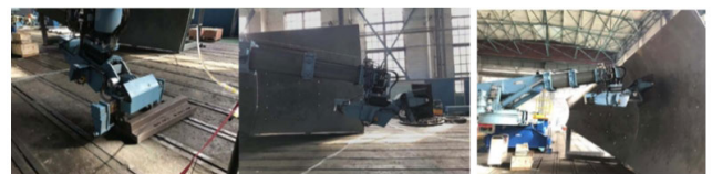
FIGURE 16. The process of grab, transport, and placement of the workpiece.
