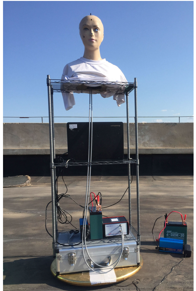
FIGURE 1. Rotating manikin with spectrometer, from top to bottom: a manikin head, a stand, and a turntable base.
