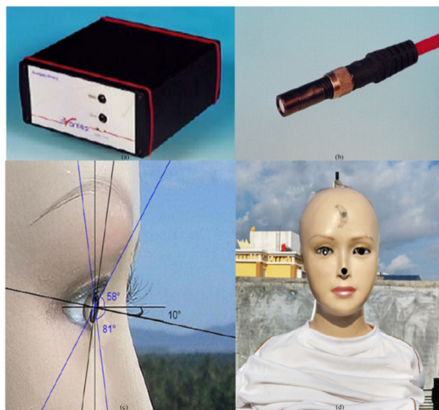
FIGURE 2. Spectrometer (a), detectors (b), angle (c) and position (d) of the manikin head.
