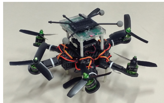
FIGURE 1. Fully actuated hexarotor aerial vehicle used in the experiment. Each rotor is tilted and fixed so that the vehicle can generate force and torque in every direction and around any axis.
