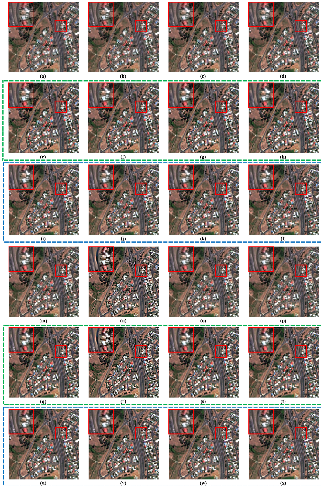
FIGURE 3. Fusion images with and without restoration on the GeoEye-1 data set at reduced scale: (a) HPF; (b) SFIM; (c) ATWT; (d) AWLP; (e) restored HPF 1; (f) restored SFIM 1; (g) restored ATWT 1; (h) restored AWLP 1; (i) restored HPF 2; (j) restored SFIM 2; (k) restored ATWT 2; (l) restored AWLP 2; (m) MTF-GLP-HPM; (n) MTF-GLP-CBD; (o) MF-HG; (p) FE-HPM; (q) restored MTF-GLP-HPM 1; (r) restored MTF-GLP-CBD 1; (s) restored MF-HG 1; (t) restored FE-HPM 1; (u) restored MTF-GLP-HPM 2; (v) restored MTF-GLP-CBD 2; (w) restored MF-HG 2; (x) restored FE-HPM 2.
