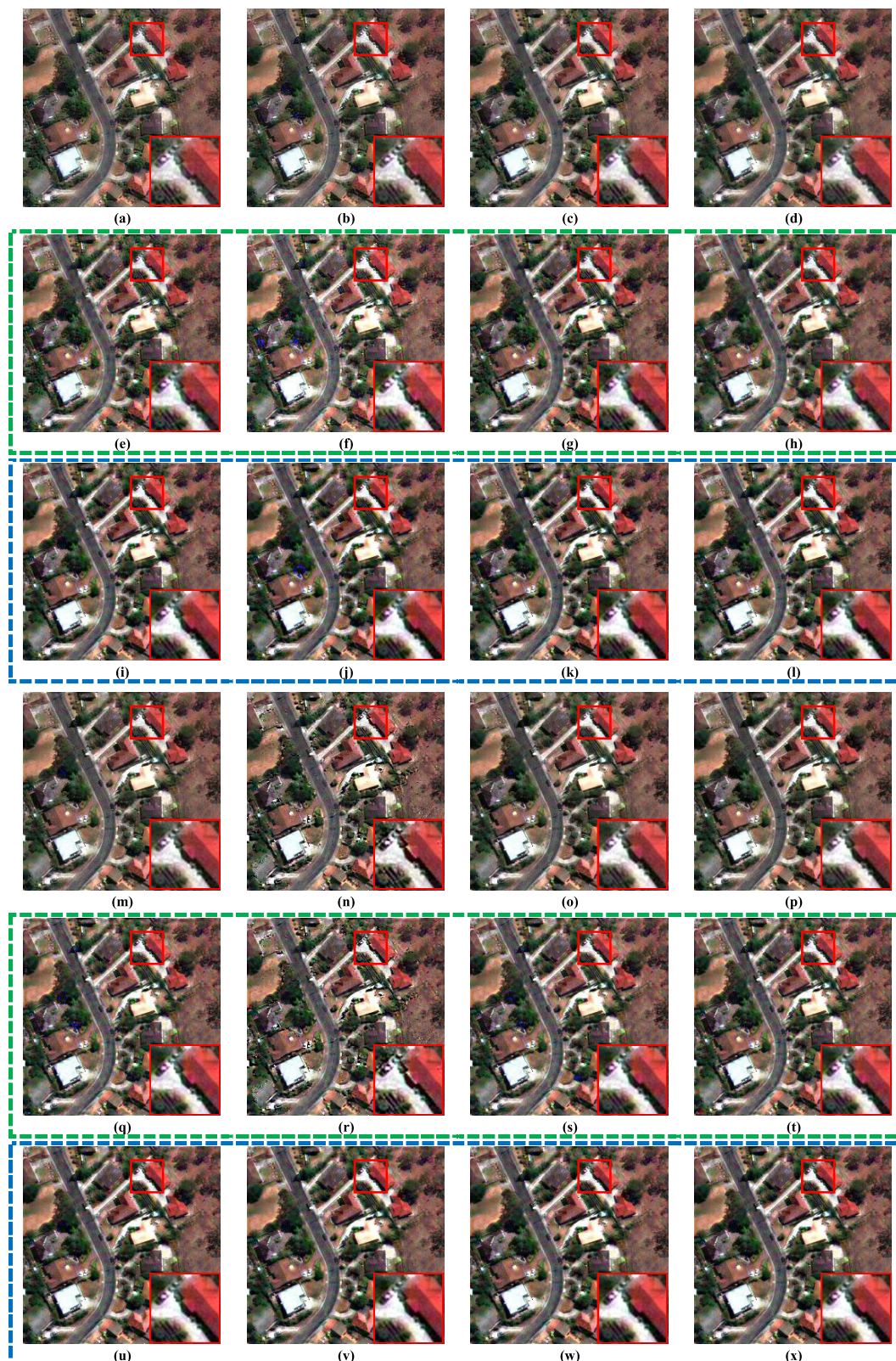
FIGURE 5. Fusion images with and without restoration on the GeoEye-1 data set at full scale: (a) HPF; (b) SFIM; (c) ATWT; (d) AWLP; (e) restored HPF 1; (f) restored SFIM 1; (g) restored ATWT 1; (h) restored AWLP 1; (i) restored HPF 2; (j) restored SFIM 2; (k) restored ATWT 2; (l) restored AWLP 2; (m) MTF-GLP-HPM; (n) MTF-GLP-CBD; (o) MF-HG; (p) FE-HPM; (q) restored MTF-GLP-HPM 1; (r) restored MTF-GLP-CBD 1; (s) restored MF-HG 1; (t) restored FE-HPM 1; (u) restored MTF-GLP-HPM 2; (v) restored MTF-GLP-CBD 2; (w) restored MF-HG 2; (x) restored FE-HPM 2.
