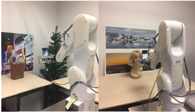
FIGURE 2. Robotic arm pointing the camera at different test scenes.
