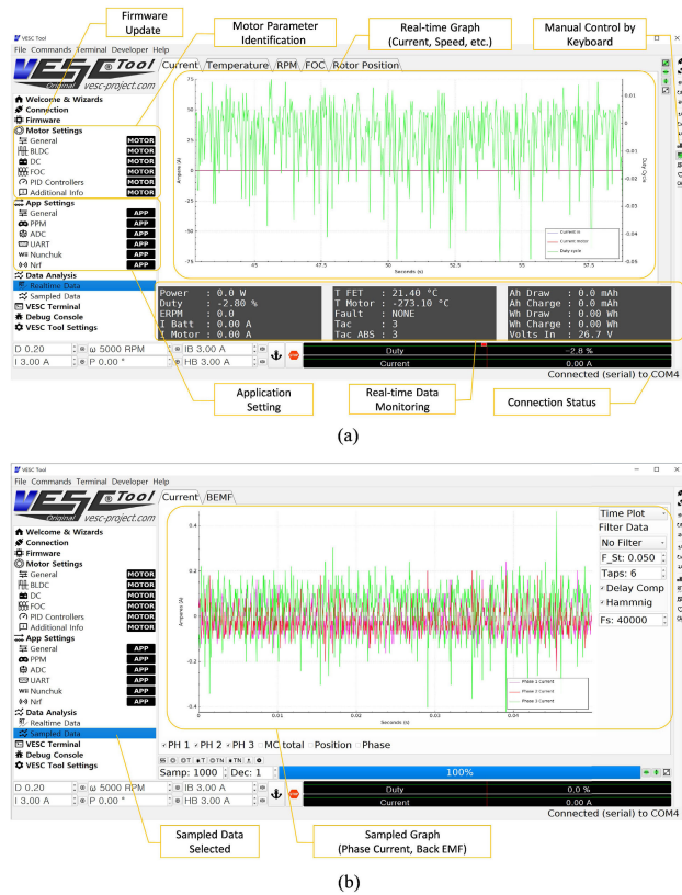
FIGURE 1. VESC-Tool GUI: (a) Real-time data view and general description of VESC-Tool and (b) Sampled data view.
