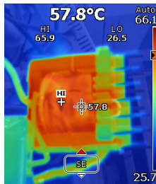
FIGURE 15. Thermal image of the prototype LHFGT using Fluke Ti200 after 35 minutes of continuous operation under 200W load with natural convection with \Delta T_r = 40.4^\circ\text{C} .
