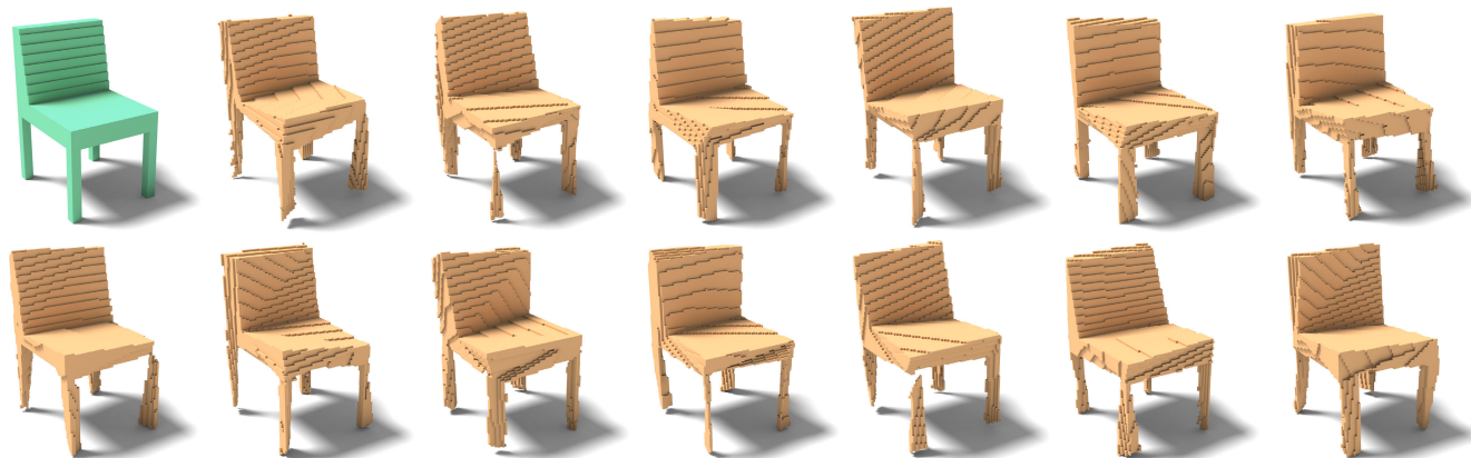
FIGURE 9. A series of random vertex displacements for dataset augmentation, with a uniform distribution limited to the 5% of the voxel space width.
