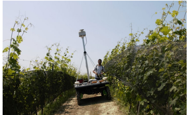
FIGURE 14. Testbed used in vineyard, with GNSS-based reference system mounted on a pole to gain good visibility of the sky.
