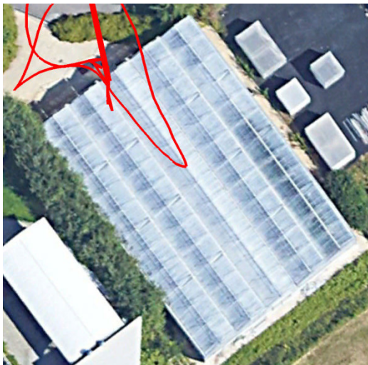
FIGURE 23. Position estimated by the GNSS Reference Receiver overlapped to an orthophoto of the greenhouse.
