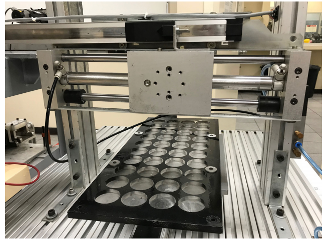
FIGURE 11. Mechanical system with a pneumatic actuator (experiment).
