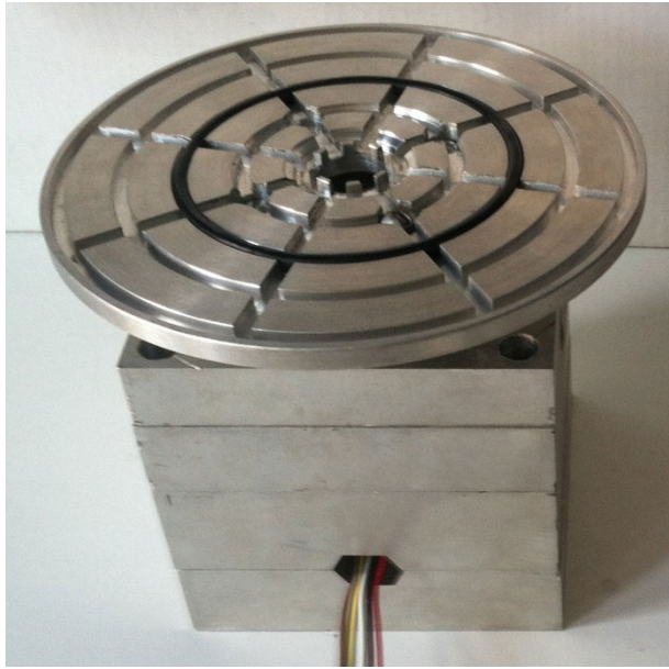
FIGURE 1. Motor housing with spinning disk.
