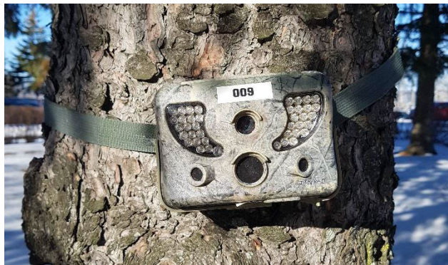
FIGURE 2. Example of an installed SpyPoint TinyHD camera.
