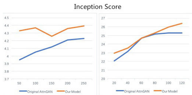
FIGURE 4. The inception scores of our method (i.e., rdAttnGAN2) and the original AttnGAN at different epochs on the CUB (left) and COCO (right) test sets.
