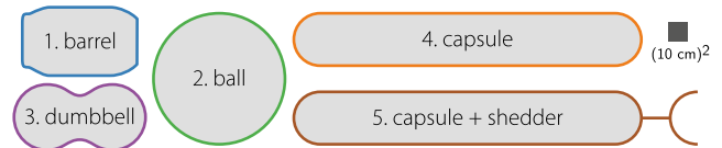
FIGURE 3. Schematic side view (to scale) of the objects used.
