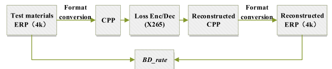
FIGURE 12. The test procedure with loss compression coding.
