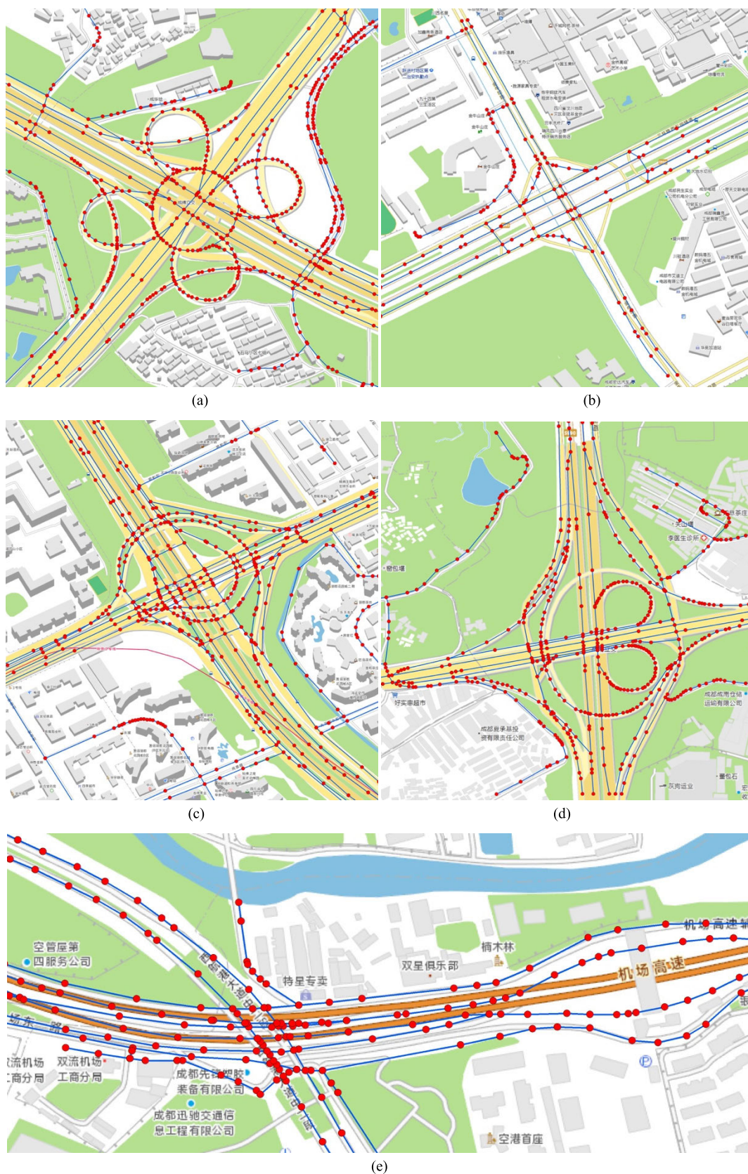
FIGURE 7. GPS data used for testing in Chengdu, Sichuan, China. This consists of five areas, including Chengmian Flyover (a), Jinniu Flyover (b), Wuhou Flyover (c), Chengnan Flyover (d), and Shuangliu Airport (e). The red dots represent GPS track points and the blue lines represent GPS track lines, which are superimposed on the road map.
