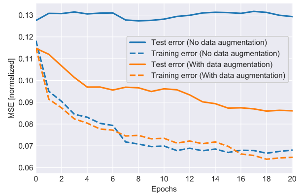
FIGURE 13. Example of the test error with and without data augmentation applied (shown in solid). The training error is shown as the dashed line for both approaches.
