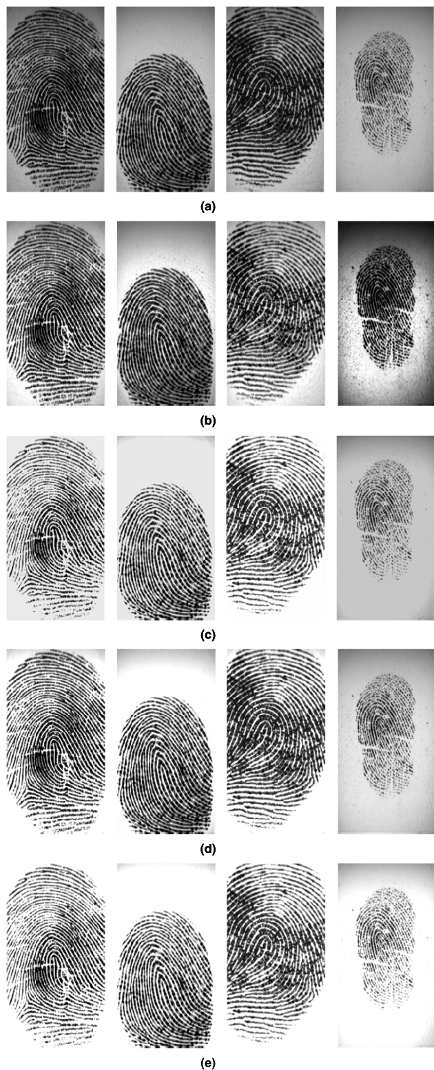
FIGURE 6. Some samples results of different enhancement approach on FVC2002 DB2-A fingerprint database. (a) The original images. (b) HE images. (c) Sharma and Dey method. (d) Wang et al. method. (e) Our proposed method.
