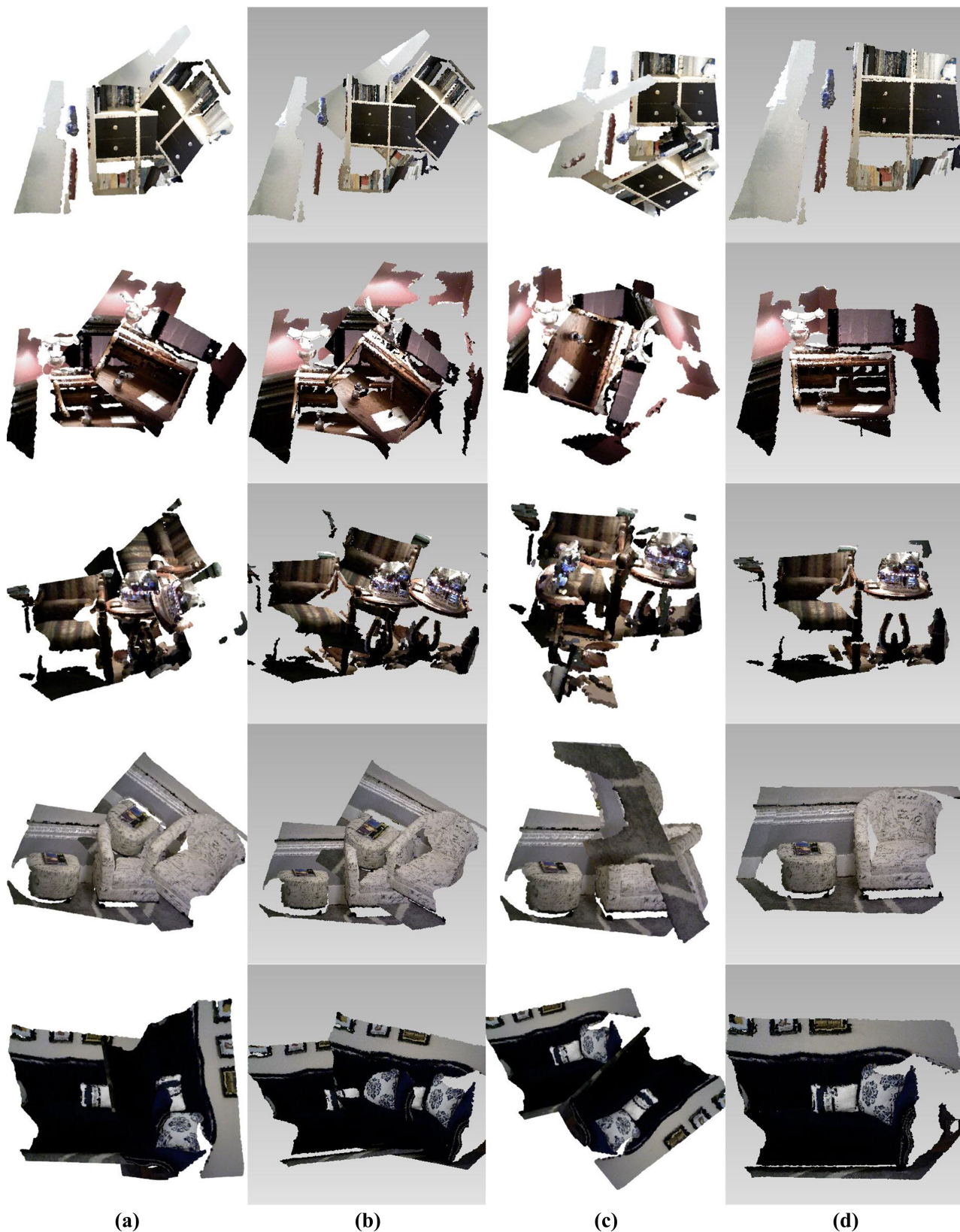
FIGURE 4. Comparison of registration results using Indoor Lidar-RGBD Scan Dataset. (a) Original point cloud data. (b) Registration result of ICP algorithm. (c) Registration result of CPCRR algorithm. (d) Registration result of our algorithm.
