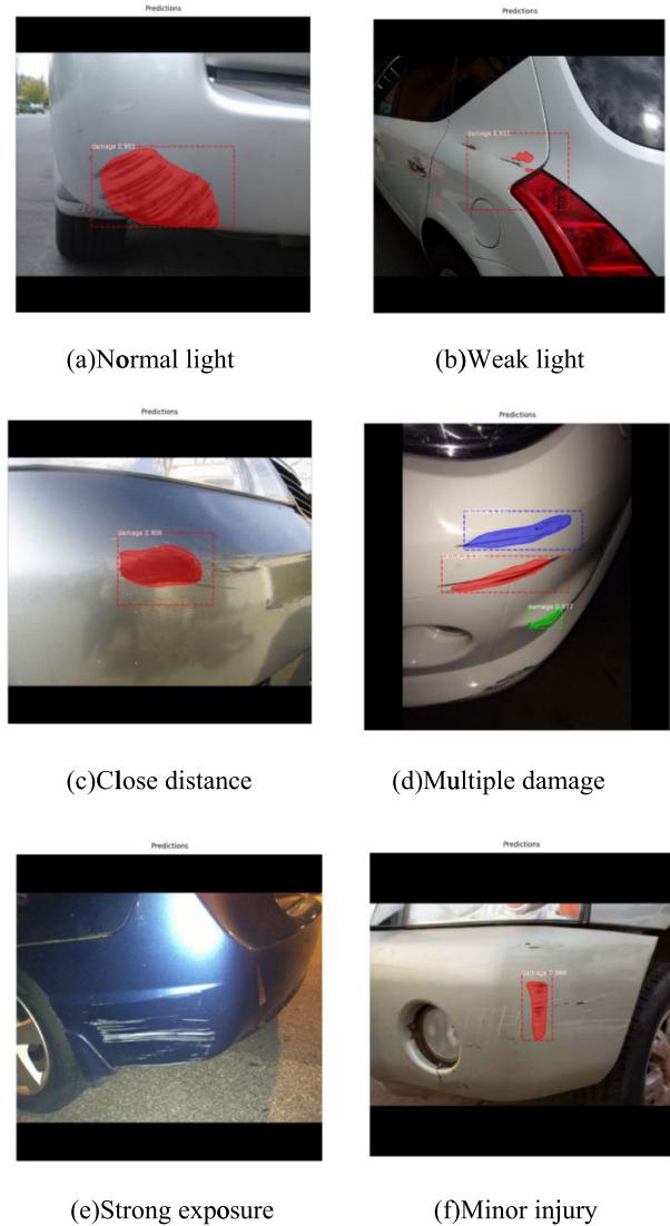
FIGURE 10. Vehicle damage detection result based on Mask RCNN algorithm.
