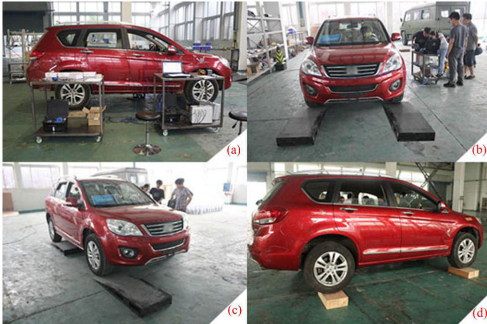
FIGURE 11. Full vehicle drop test (a) test set up; (b) front axle drop test; (c) right side drop test; (d) all wheels drop test.
