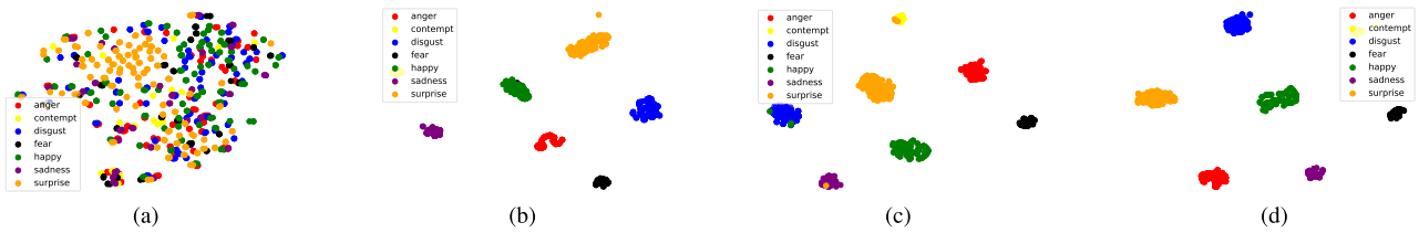
FIGURE 6. Visualization results on CK+ dataset. (a) Visualization of original input data. (b) Visualization of output features learned using the OSE method. (c) Visualization of features learned using the PS method. (d) Visualization of features learned using the PSE method. The data points were automatically grouped by PI&DML model.
