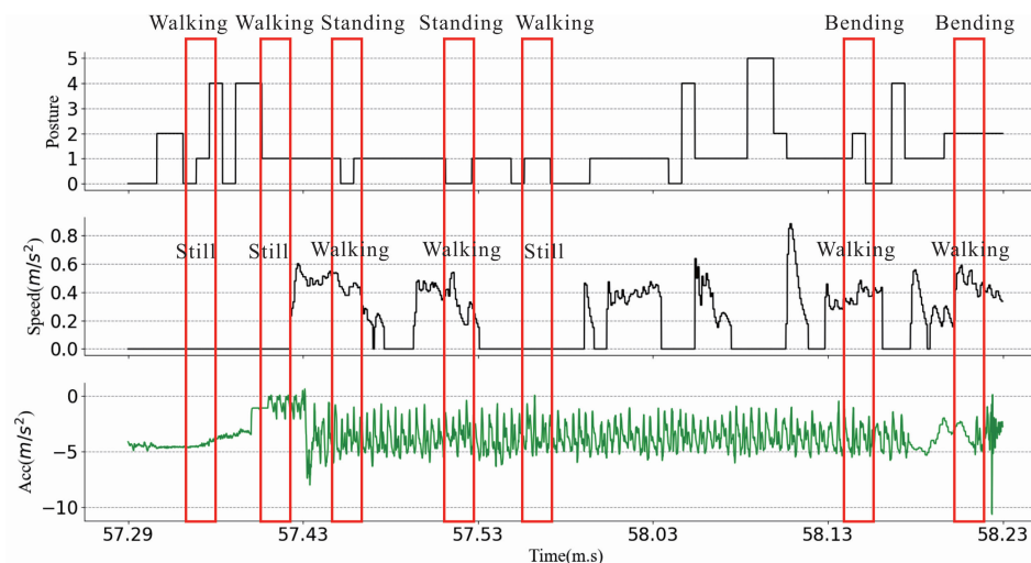
FIGURE 9. Problematic areas of posture estimation in identifying standing and walking. Red rectangles indicate the misclassification areas. The speed estimation can help in refining the estimated postures. Time axis is shown in minute.second.
