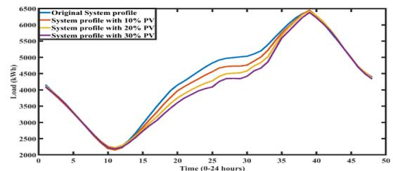
FIGURE 10. Forecasted original and PV embedded system profiles.
