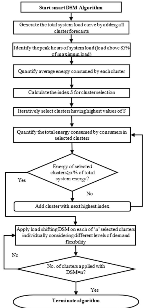
FIGURE 4. Smart DSM and consumer selection algorithm.
