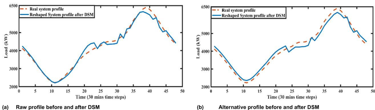
FIGURE 15. Reshaped system profiles using raw and alternative profiles (Case II, 10 clusters, 15% demand flexibility, 10% PV).
